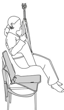
**3** Attach the loops to the spreader bar and lift.
